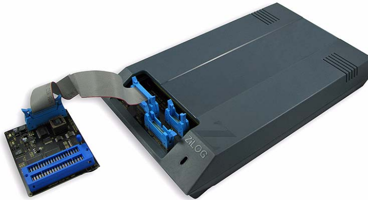
Figure 5. OTP Programming Adapter (Included with Crimson ICE)
